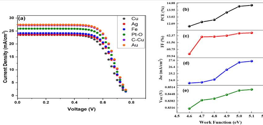
Figure 8. (a) J-V comparison at different values of work function, (b) PCE, (c) FF, (d) Jsc, and (e) Voc.
