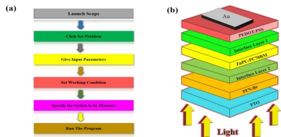
Figure 1. (a) Basic steps for numericalization SCAPS-1D, and (b) A diagrammatic representation of the intended DSSC structure
