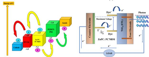
Figure 2. (a) HOMO-LUMO band diagram of the proposed DSSC, and (b) Schematic of operation principle of DSSC.
