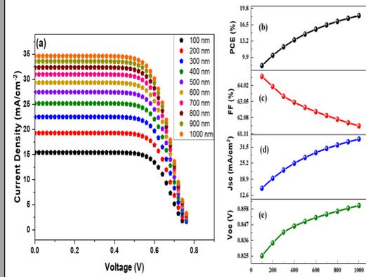
Figure 4. (a) J-V comparison at different values of thickness, (b) PCE, (c) FF, (d) Jsc, and (e) Voc in relation to photoactive layer thickness.
