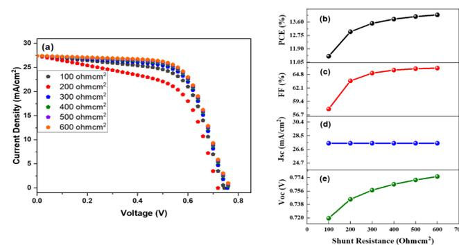
Figure 6. (a) J-V comparison at different values of Shunt resistance, (b) PCE, (c) FF, (d) Jsc, and (e) Voc in relation Shunt resistance.
