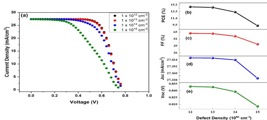
Figure 7. (a) J-V comparison at different values of defect mobility, (b) PCE, (c) FF, (d) Jsc, and (e) Voc
