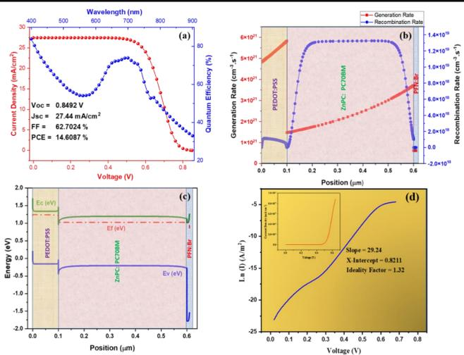
Figure 3. (a) J-V and QE curve of the intended device (b) Generation and recombination rate of photogenerated carriers in device (c) Energy band structure of purposed device, and (d) Ln (I) vs Voltage (Inset represents Dark J-V Measurement).
