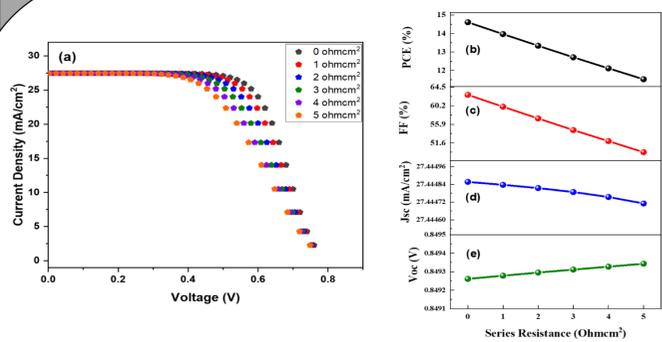
Figure 5. (a) J-V comparison at different values of series resistance, (b) PCE, (c) FF, (d) Jsc, and (e) Voc in relation to series resistance.
