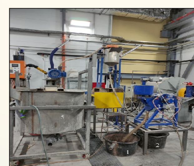
Obtaining aluminosilicate microspheres by enrichment of ash and slag waste
