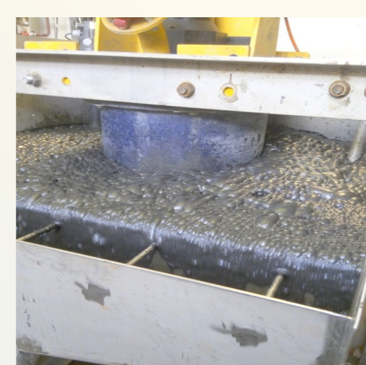
Obtaining aluminosilicate microspheres by enrichment of ash and slag waste
