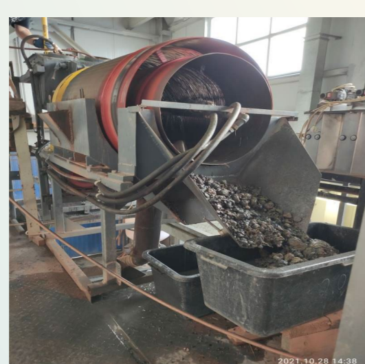
Obtaining aluminosilicate microspheres by enrichment of ash and slag waste
