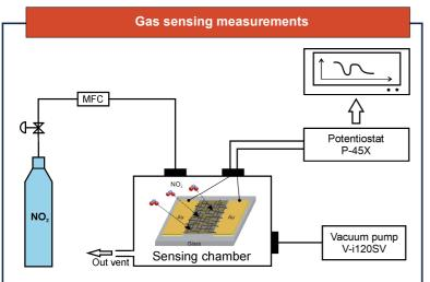
The sensory properties of the finished samples were studied on specially designed equipment, consisting of a sealed capsule, a detector with an embedded gas-sensitive element, a target gas cylinder, a pressure-reducing valve, a personal computer, and a potentiostat for controlling a given voltage and measuring current. The tests were carried out at room temperature and relative air humidity of 45%. Nitrogen dioxide was used as the target gas.
