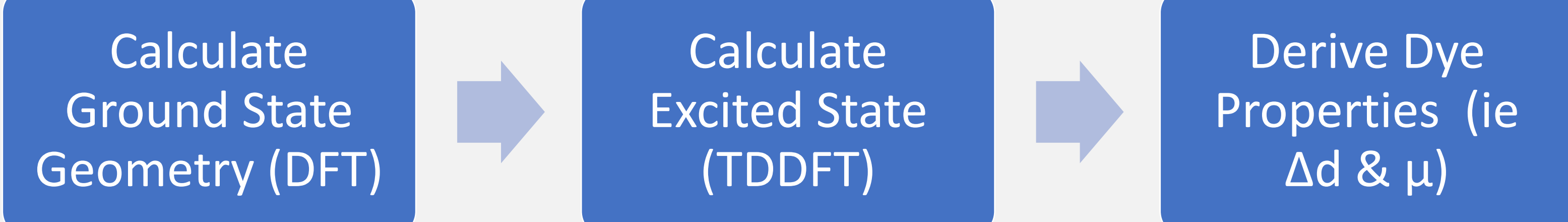
Fig 2: General workflow for deriving dye properties with DFT and TDDFT
